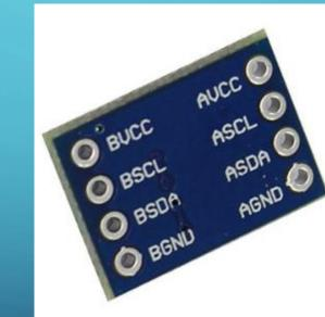
USPRO® IIC I2C Level Converter with pins conversion Module Compatible With 3-5V System for Arduino Sensor by USPRO Be the first to review this item
